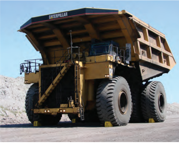
Four Monster wheel chocks, model MC3011 used on a 400-ton CAT 797
