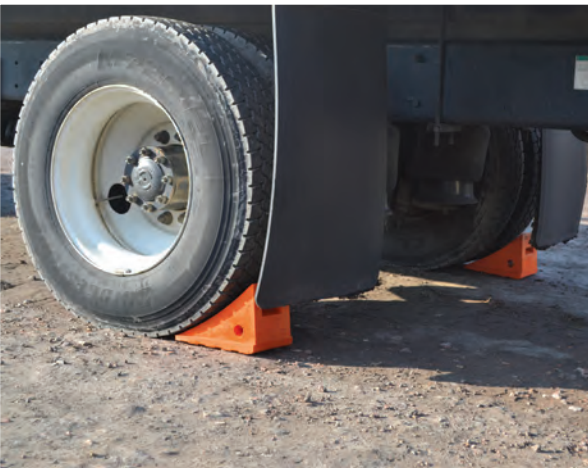
Monster Urethane Chock model UC1500-6 being used on a mine support truck
