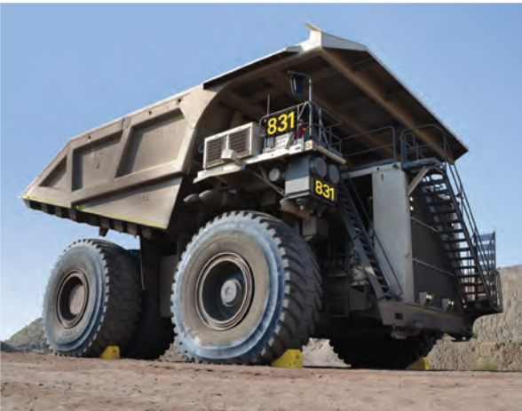
Four Monster wheel chocks, model MC3011 used on a 400-ton Liebherr haul truck
