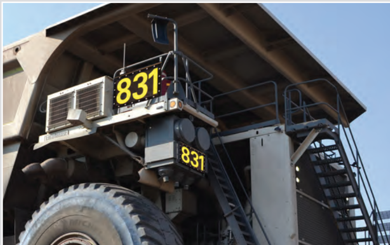
AID™ Rectangular Vehicle Identification Light on a 400-ton mine haul truck.
