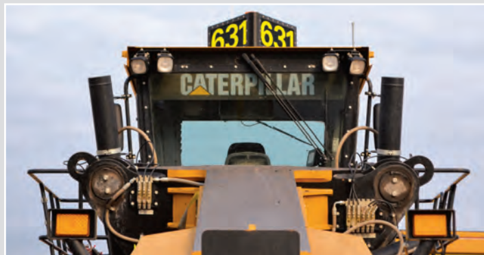
AID™ Triangular Vehicle Identification Light on the top of a grader.
