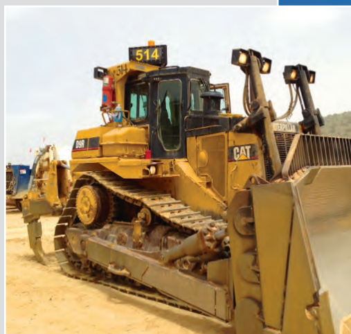
AID™ Triangular Vehicle Identification Light on a dozer.
