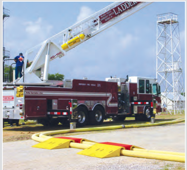
Diamondback Hose Bridges in use at a fire training facility
